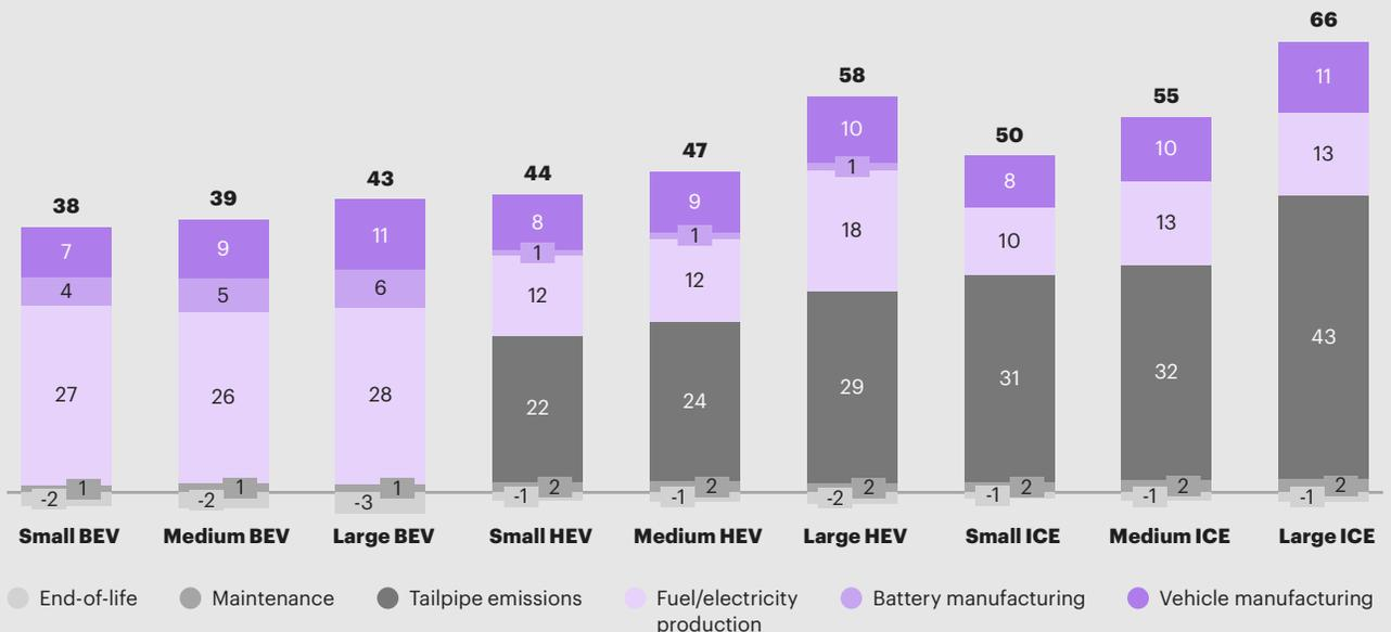
Notes: BEV is battery electric vehicle. HEV is hybrid electric vehicle. ICE is internal combustion engine. Numbers may not resolve due to rounding.
