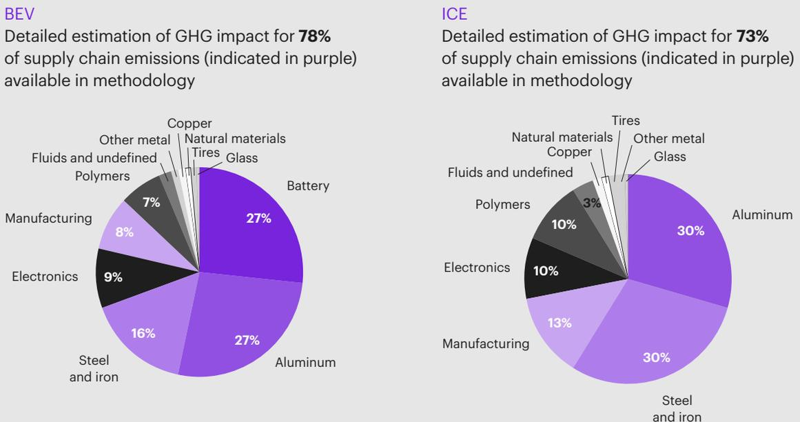
Notes: EV is electric vehicle. BEV is battery electric vehicle. ICE is internal combustion engine. GHG is greenhouse gas. Sources: Polestar LCA report; Kearney analysis
