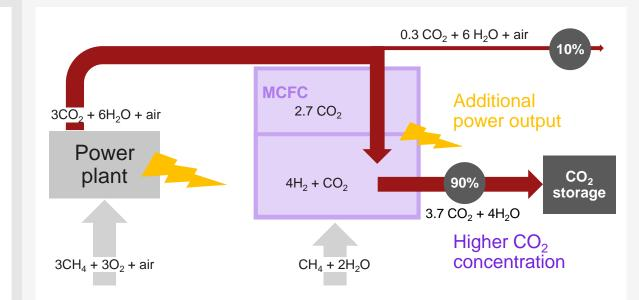
Power output: +50% to +200% (depending on CO<sub>2</sub> capture intensity) Estimated carbon intensity:~40 to 25g CO<sub>2</sub>/kWh
