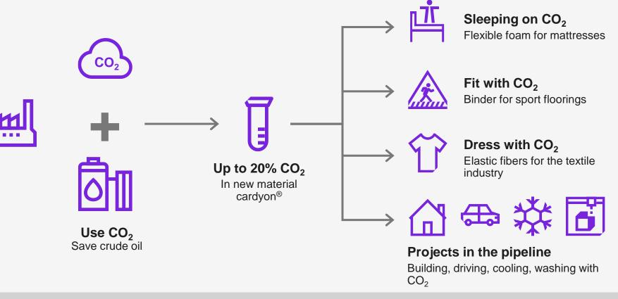
Cardyon<sup>®</sup> is manufactured with an innovative method that uses a new catalyst, which causes the  $CO_2$  to react with propylene oxide to produce certain plastic components known as polyols. This results in a new type of polyols with a  $CO_2$  share of up to 20 percent substituting crude oil feedstock completely.
