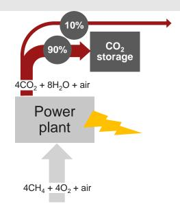
Power output: 400MW for a 500MW plant Estimated carbon intensity: ~60g CO<sub>2</sub>/kWh
