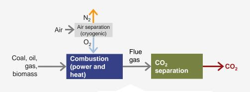
Flue gas mainly consists of  $CO_2$  and  $H_2O$  which are separated by condensing water
